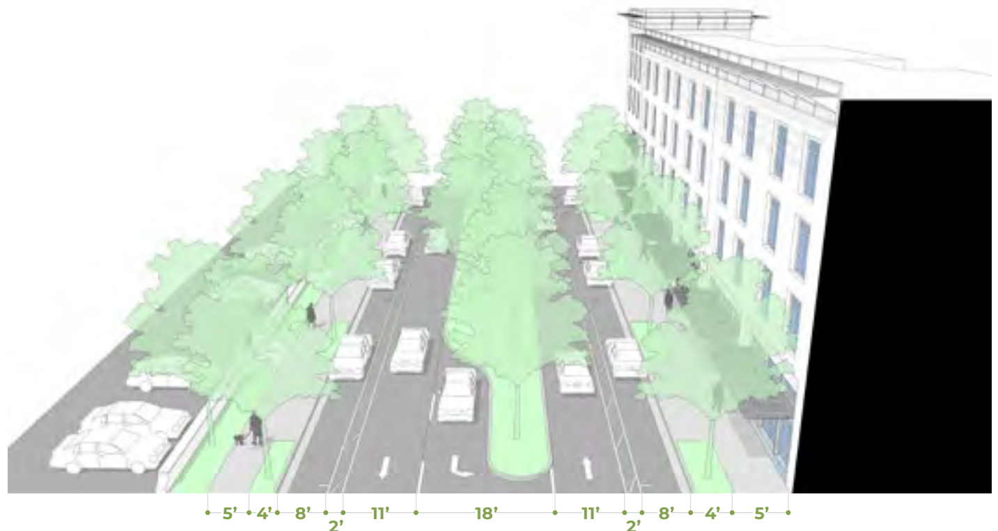
Figure 4-4 Future Main Street Cross Section (Central Avenue to 1st Street)
