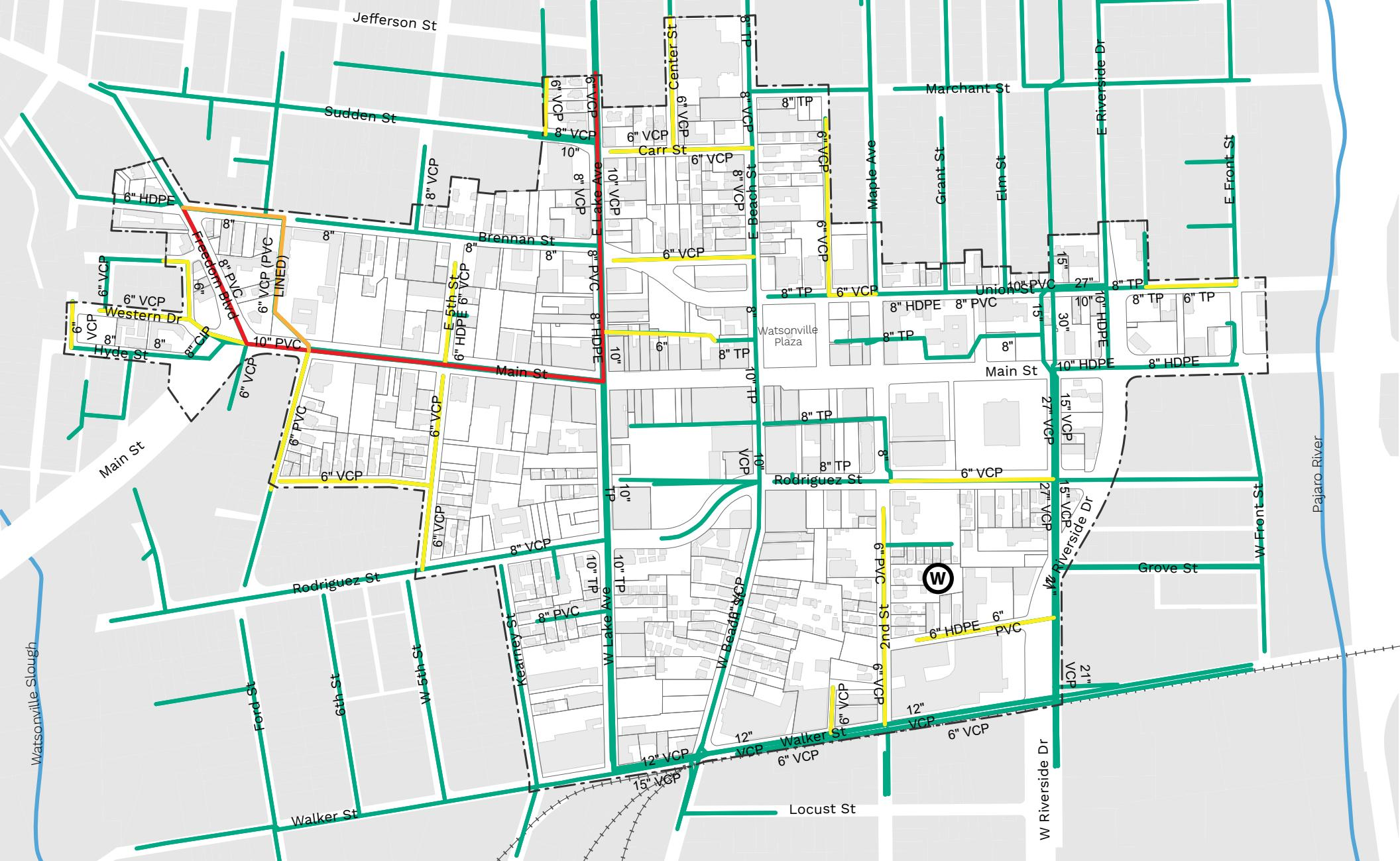
**FIGURE 8-2 SANITARY SEWER: EXISTING FACILITIES & RECOMMENDED IMPROVEMENTS**
