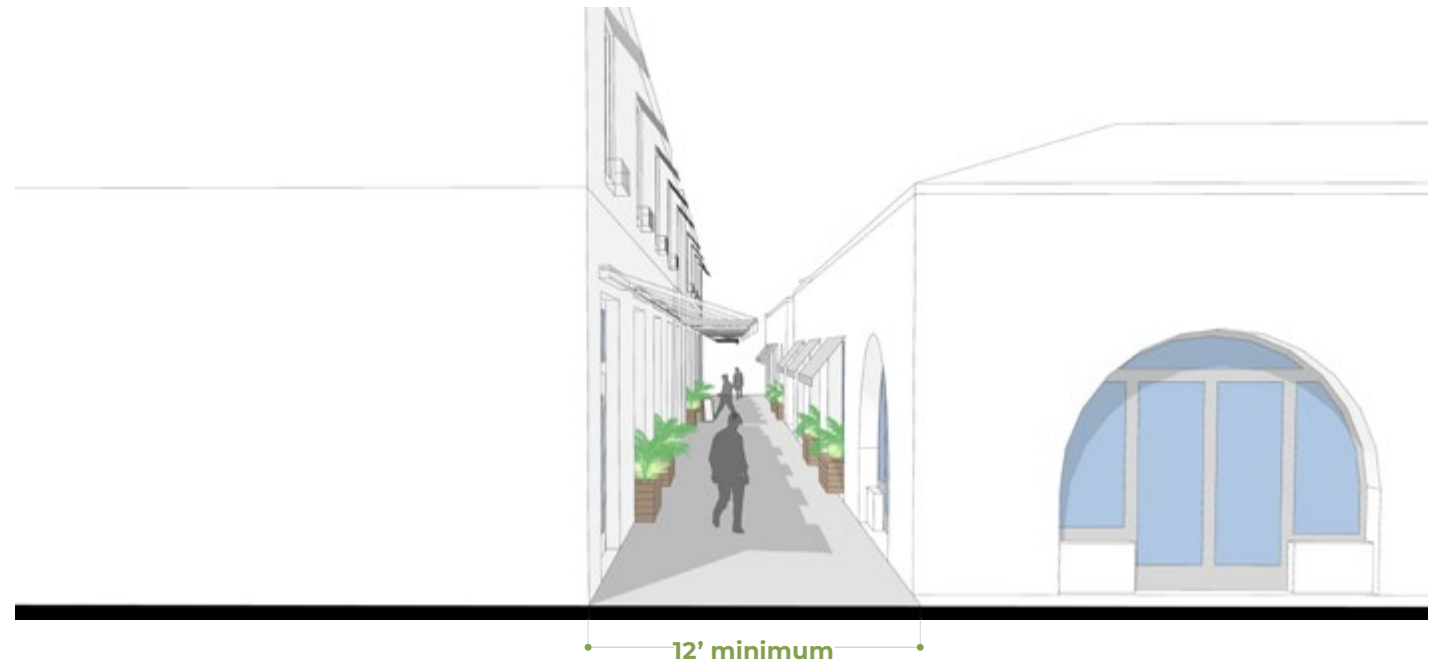
Figure 4–8 Future Paseo Cross Section
