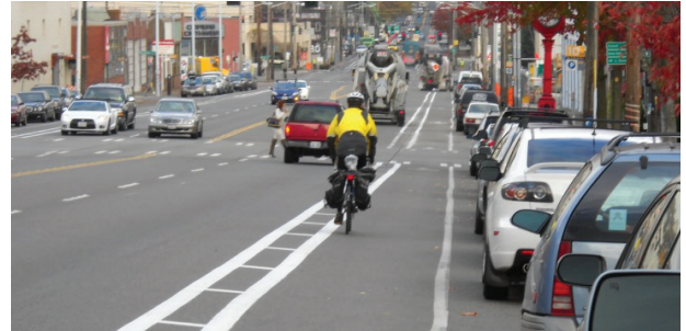
Figure 37 | Bike Lane with Buffer
