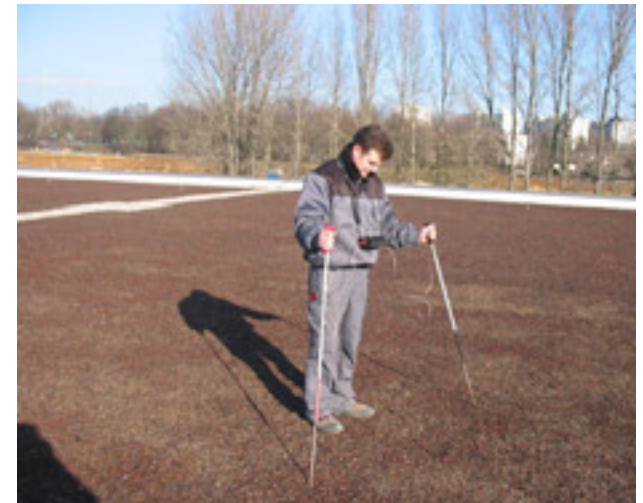
Figure 4.2 Electronic leak detection on a green roof
