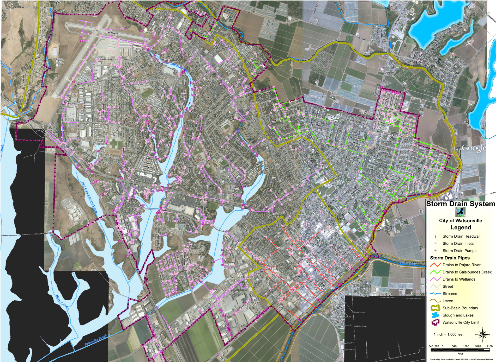
Figure 1.1 Storm Drain System of Watsonville, colored by subwatershed. Modified from City of Watsonville Green Roof Report, City of Watsonville CA
